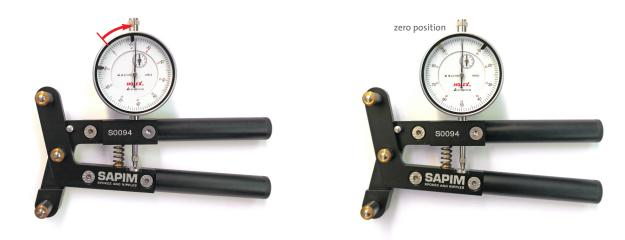
Press the handles together and put the tensiometer on the spoke so that the spoke lays between the bearings (see picture).
