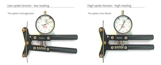
The tensile force of the spoke is indirectly measured by the deformation of the spoke.
